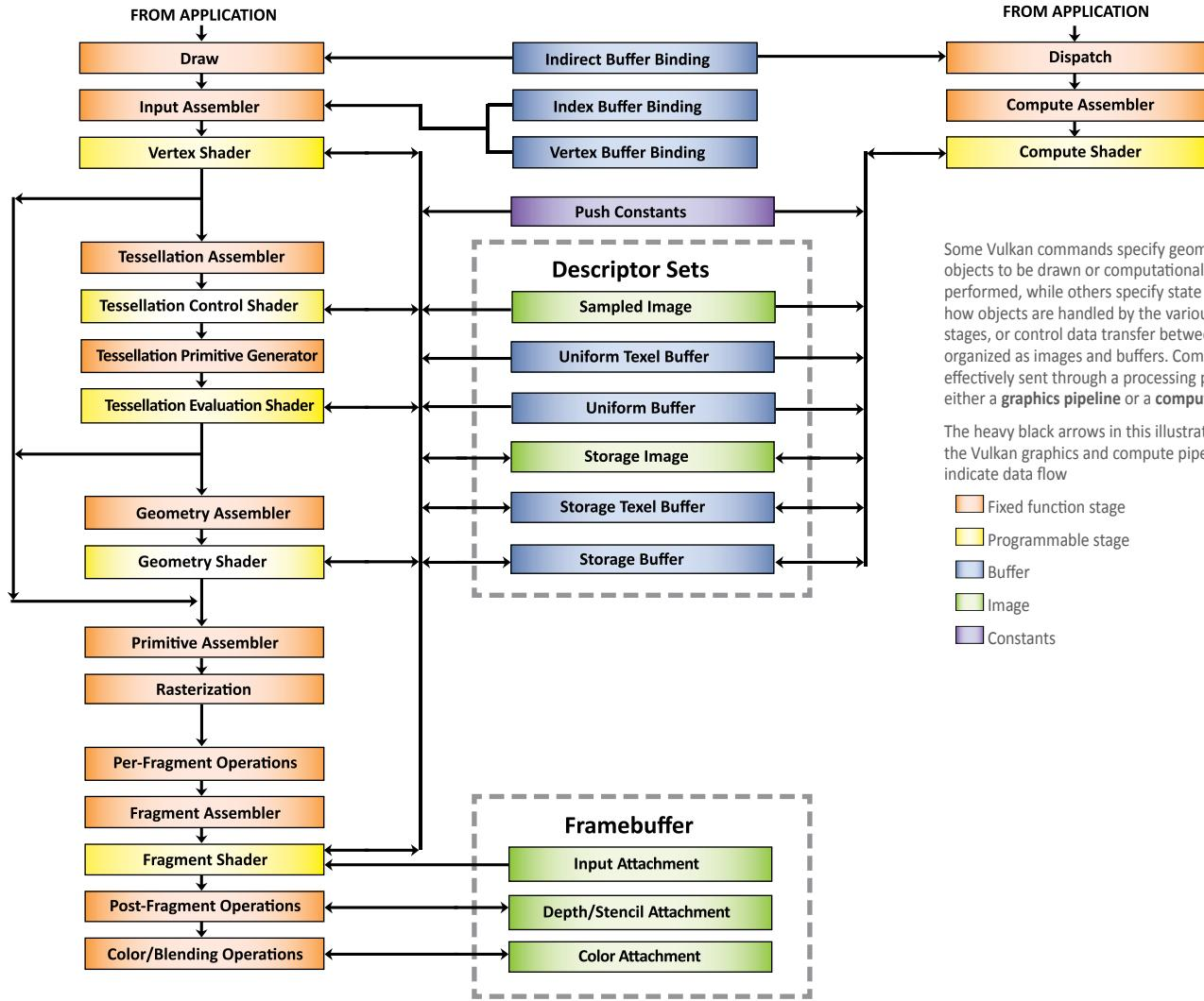
Some Vulkan commands specify geometric objects to be drawn or computational work to be performed, while others specify state controlling how objects are handled by the various pipeline stages, or control data transfer between memory organized as images and buffers. Commands are effectively sent through a processing pipeline, either a graphics pipeline or a compute pipeline.
